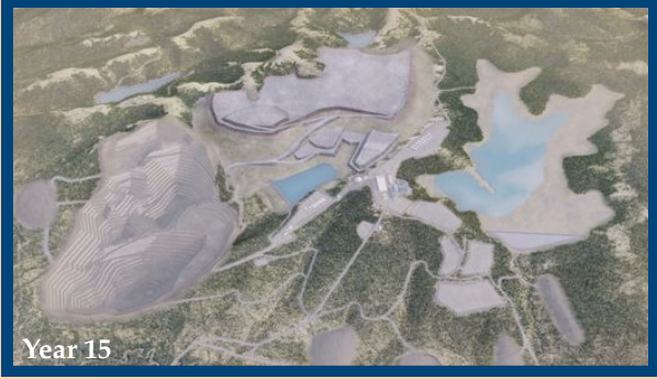
Year 15: Pit, waste treatment facility (tailings storage) & waste rock facility at about half of ultimate extent. Concurrent reclamation is shown.
